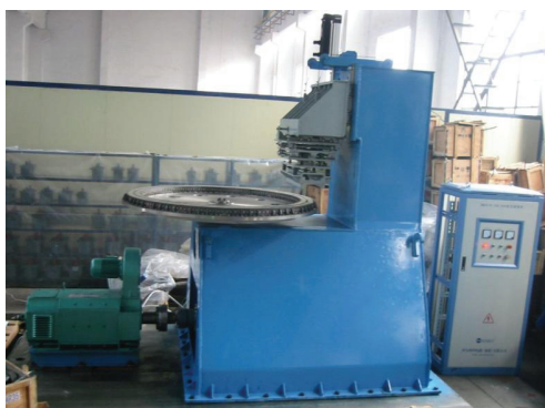
Fig. 29. The photo of the airframe of the HTS Maglev dynamic test system SCML-03: 3.3 m long, 2.4 m wide and 3.15 m high With a total weight of 13.95 t
