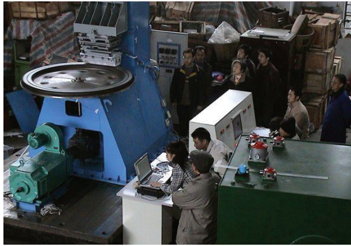
Fig. 30. The measurement scene of the HTS Maglev dynamic test system. On the right side is the control desk
