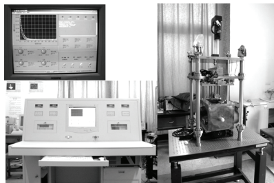
Fig. 15. Photo of the SCML-02 HTS Maglev measurement system: Levitation force measurement interface (top left corner); Console control desk (under left corner); Experiment system (right).
